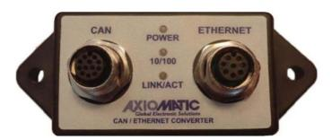
The Converter has one tri-color LED for Power and 2 green LEDs for Ethernet. It can operate with DC power between 9 to 36 V. Surge, reverse polarity, overvoltage, and undervoltage protection is provided.
