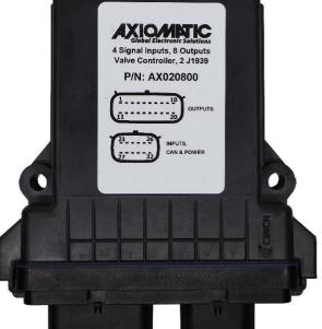
The device interfaces with 2 SAE J1939 CAN networks using auto-baud-rate detection and utilizes a Wake-on-CAN function to save on power.
