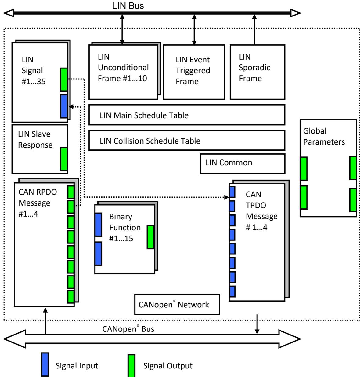
The actual connections between signal inputs and outputs are defined by the configuration parameters.
