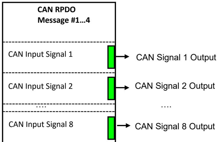
Figure 14. CAN Input Signal Function Block
