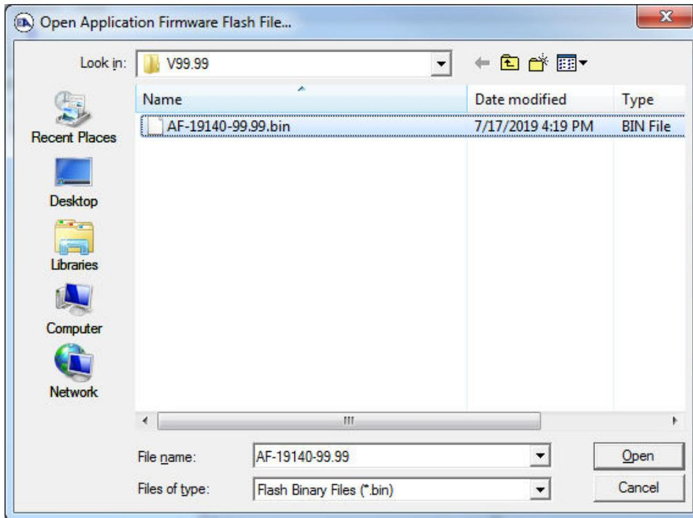
7. Open the flash file and start flashing operation by pressing the *Flash ECU* button.
