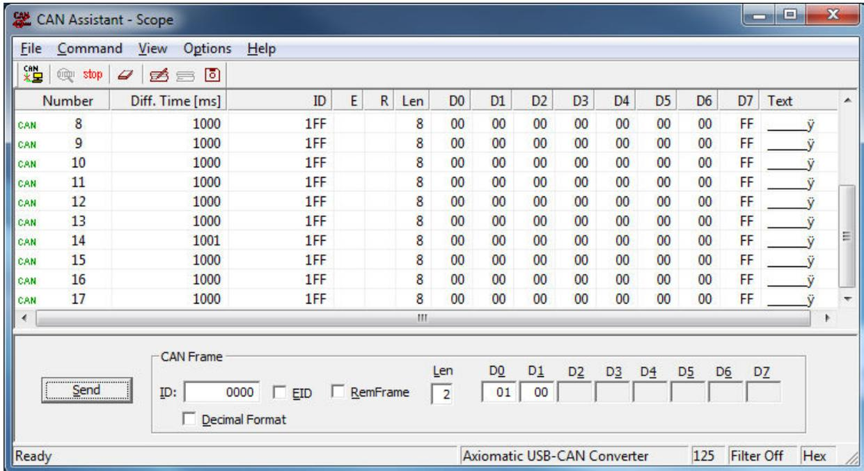
2. Configure the LIN Common function block (index 2001h, 2002h, 2003h) to start the LIN bus communication. This can be done by sending a CAN message, for example, to the index 2002h as following:
