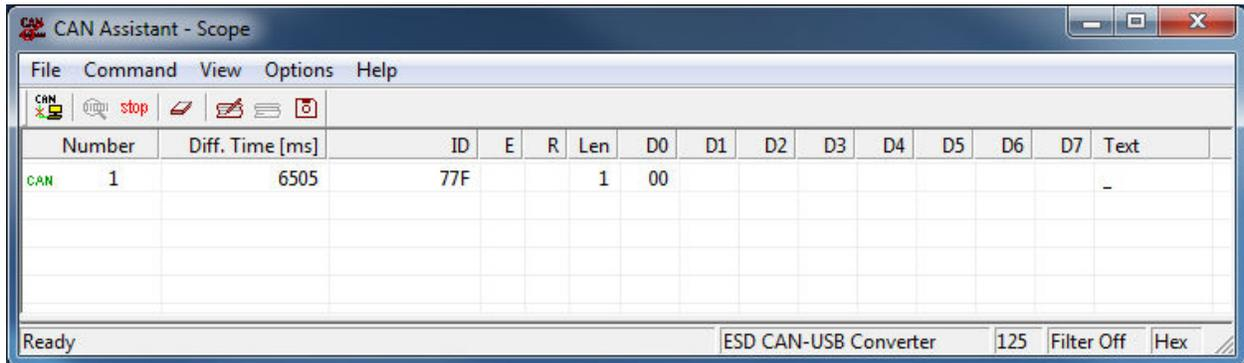
4. Set the CANopen® object 0x55AA to 1 using SDO protocol. To do so, send the following message using CAN Assistant – Scope:
