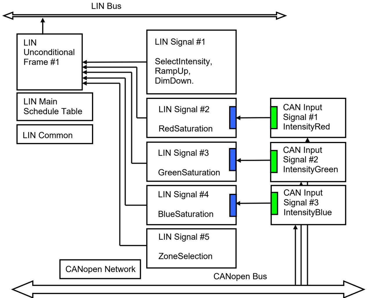
Figure 16. Block Diagram of the Example Converter Configuration
