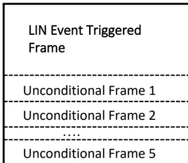
Figure 7. *LIN Event Triggered Frame* Function Block
