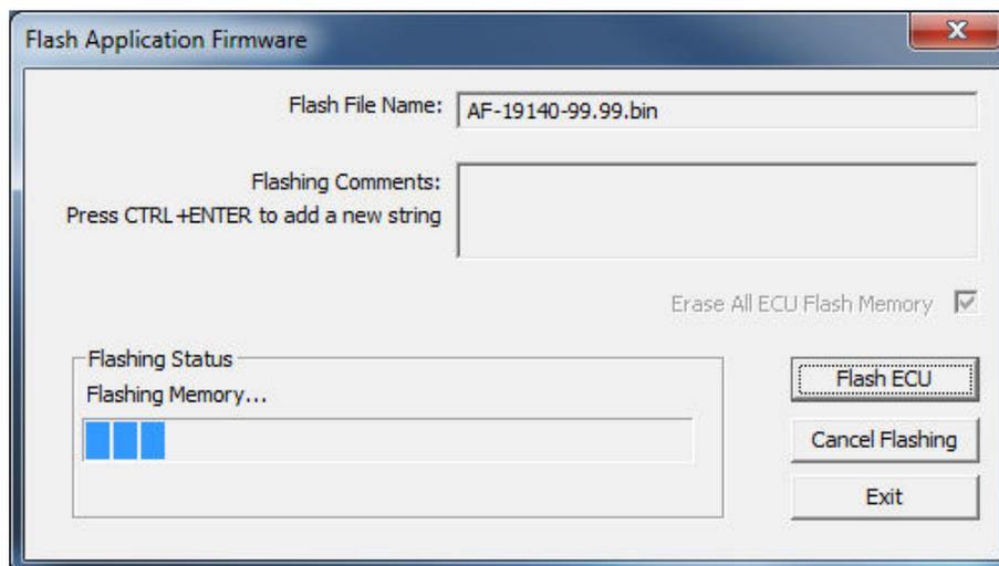
9. When flashing is done, reset the ECU.
