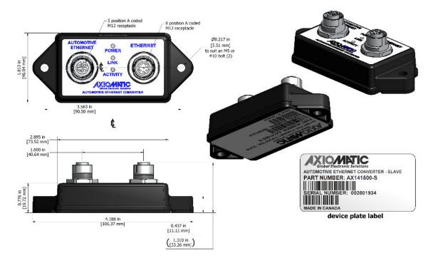
Figure 2.0. Dimensional Drawing – AX141500-S
