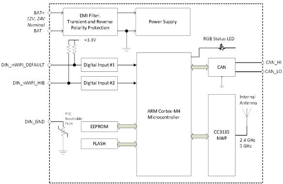
Figure 1.0 – Block Diagram
