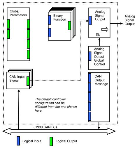
As an example, the logical output of the CAN Input Signal functional block is connected to the logical input of the Analog Signal Output functional block, providing a direct path for the CAN input signal to the controller signal output.
