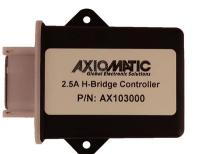
AX103000: Compact H-Bridge Controller with 3 Universal Inputs and 2 Outputs
