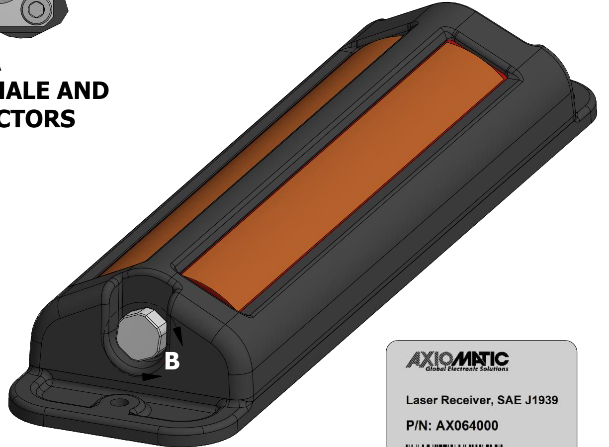
DETAIL B POLYVENT VALVE
